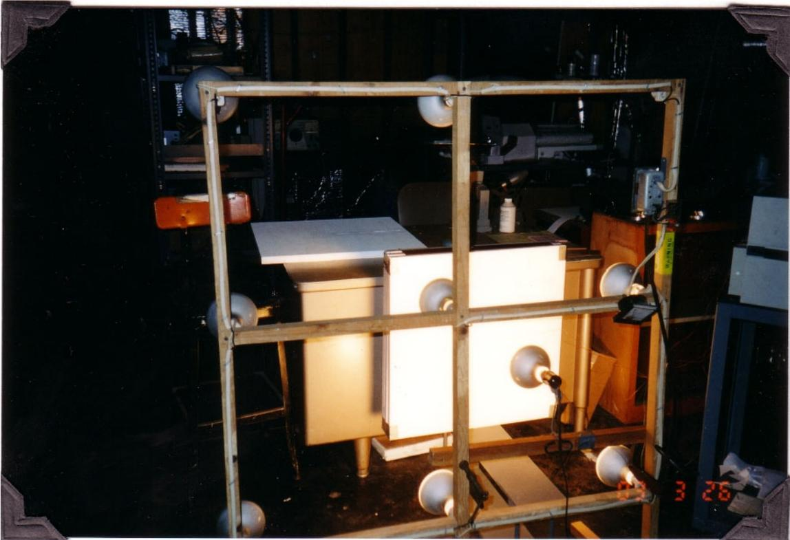
Photograph of the solar lamp array and Insuladd painted wall panel
