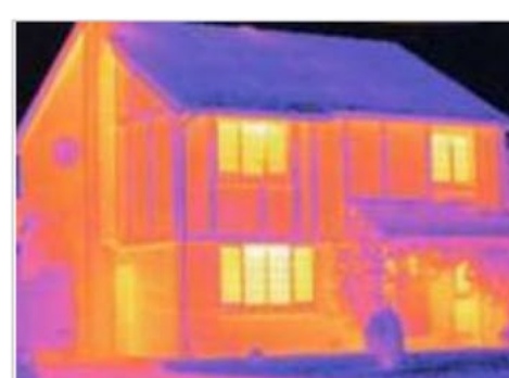
Thermographic image shows areas of high heat loss (red and yellow) from a home. The blue roof indicates good insulation and little heat loss. Image Credit: The Insuladd Company
